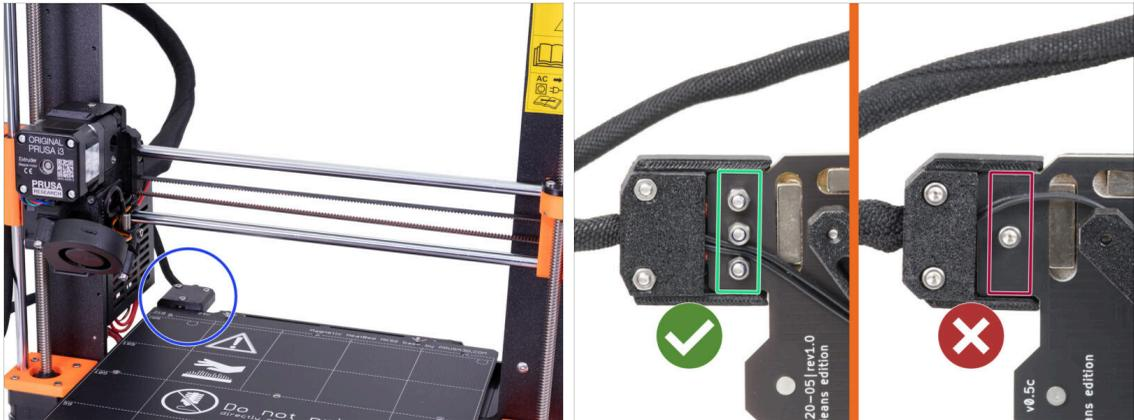
⚠ **The upgrade from MK3S/MK3S+ to MK3.5S is compatible with the heatbed that has screwed power cables.**
