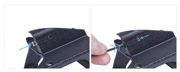
Insert the M3nS nut into the External-PSU-bracket-DELTA. Using the Allen key, push the nut all the way into the printed part and align the nut with the hole in the part.
