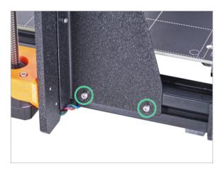
Fully tighten the screws on the printer frame support.
