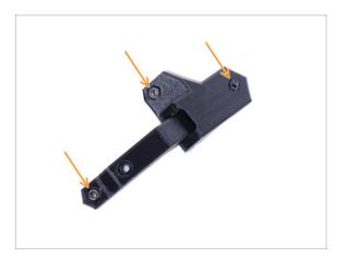
Insert three M3n nuts into each hinge assembly.
