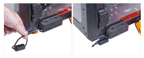
Connect the external PSU cable to the basic board from the left side.
