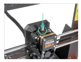
Insert and screw the Fitting QSM-M5 directly into the threaded filament hole in the extruder.
